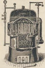
Doric Seamless Tubular Steam Boiler Sectional View
