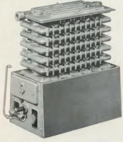
Seven-section Boiler assembled without casing and jacket. The sections and base are rugged cast iron. Sections are hydrostatically tested to rigid ASME specifications before and after assembly.
