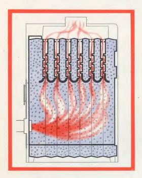
The Utica Starfire Boiler is entirely new in advanced heating design. It combines in one smartly-styled, handsomely-finished unit the two most desirable features for economical, efficient operation... vertical flue travel plus cast-iron wet-base construction!
