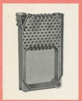
Rugged cast iron sections heat fast, hold heat longer and are rust and corrosion resistant. The patented 'Free-Floating' construction provides independent expansion of each section. A unique V-shaped, rubber-cushioned header allows boiler water to flow unrestricted between sections, equalizing boiler water temperature and assuring peak operating efficiency.
