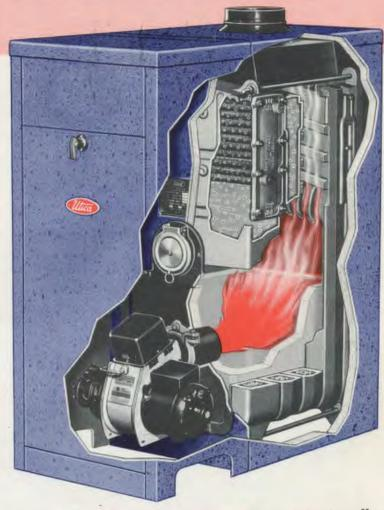
Cut away view of the Utica Starfire Boiler with extended jacket — Here you can see the construction and design features that make the Starfire Boiler so efficient and so economical to operate. Notice particularly the convenient location of the tankless heater, the slow, effective travel of hot gases as they pass around the "Slo-flo" baffles, the combustion chamber area that is completely surrounded with water for rapid and efficient heat transfer!
