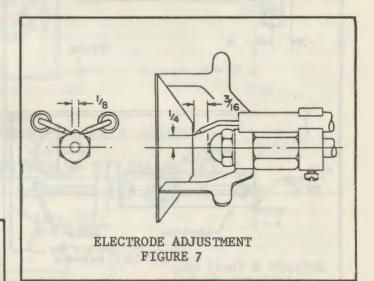
C. ADJUSTMENT PROCEDURE INITIALLY SET ALL BURNER ADJUSTMENTS MIDWAY BETWEEN MINIMUM AND MAXIMUMS SHOWN IN TABLE 3.
