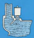
ELIMINAIRE®—A patented cost-saving feature. This built-in air eliminator is cast into the front section of all V<sub>1</sub> Series boilers to divert rising air bubbles into a tapping for connection to the expansion tank. No external device is required to separate air and water, reducing cost and installation time.
