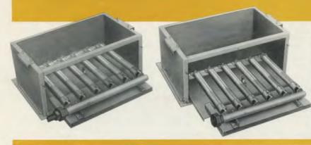
The FREEDOM 62 features a unitized burner assembly. Steel burners are factory assembled and aligned, then securely mounted on the burner tray. The entire burner assembly slides out by releasing two catches and disconnecting main gas line.
