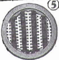
5 The grate bars are triangular in shape and revolve in pairs. Clinkers are easily ground up and discharged into the ashpit. Grate bars are heavily constructed for greatest durability.
