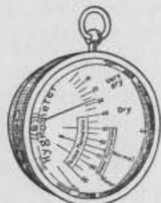
FIGURE 2. HYGROMETER USING SUBSTANCE SENSITIVE TO MOISTURE CHANGES
